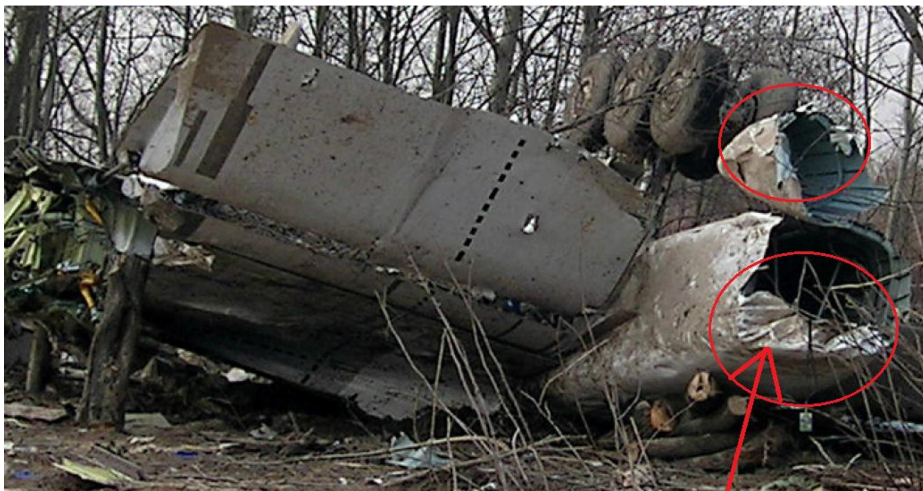
Fig. 10. The left wing root shortly after the crash. The portion shown in the pictures left side was originally facing towards the fuselage. Notice the wheels are soiled on the inwards side of both rows, but not along the entire rim, only at the small portion of the rim, that was facing downwards during the sideways sliding/turning movement of the wing piece. Also notice the end of the wheel house shows indication of being hit by an object (most likely a tree) from the wings topside during the roll movement described below.
