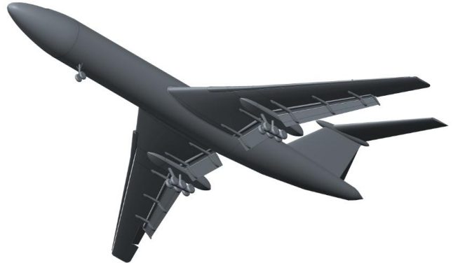
Fig. 8. Bottom view of the 3D model of the TU-154M in landing mode. Note the double slotted fowler flaps.
