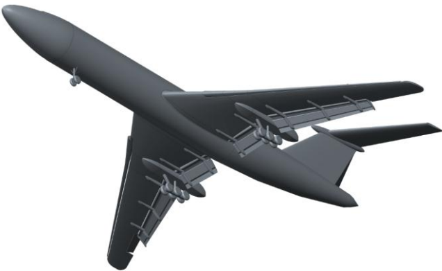
Fig. 5. Bottom view of a 3D model of the TU-154B in landing mode. Note the triple slotted fowler flaps.
