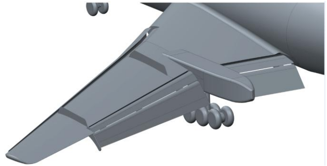
Fig. 9. Close view of a 3D model of the TU-154M in landing mode. Note the double slotted fowler flaps and extended slats towards the tip.
