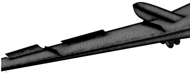
Fig. 11. Close look at the region of the aileron and outer interceptor of the right wing in the case of full pilot interaction.
